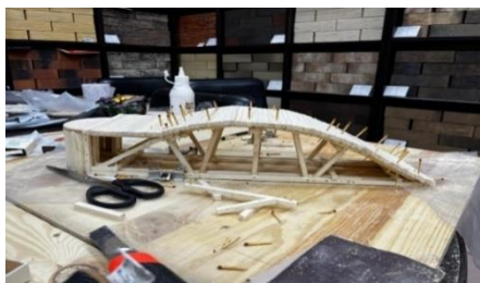
Fig. 13. Assembled Bridge Span
