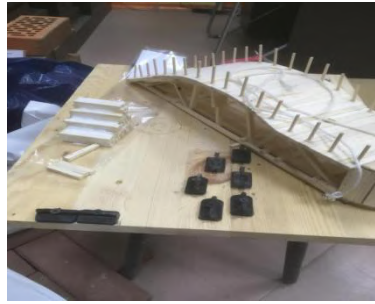
Fig. 17. Installation of Bridge Railings
