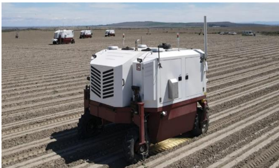
Fig. 2. Autonomous laser weeding machine Autonomous LaserWeeder [2]
