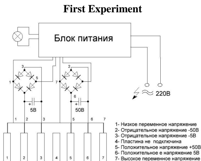
Fig. 1. Diagram of the first setup based on a printer power supply
